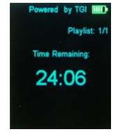
Touching any <u>arrow</u> button will change the Power Save display to the previous play screen without interrupting the program. Briefly pressing the center button will change the display to the previous play screen and pause the program, pressing the center button again will resume the play. Pressing and holding the center button until the display changes to the "Track Selection/Detail" screen stops the program. Note: Holding the center button too long will turn the MASTER KEY off.
